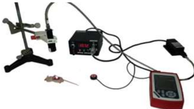
Fig 1. Red diode laser for superficial illumination. Setup of laser system.
